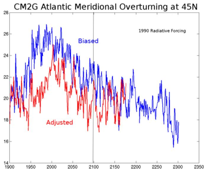
Eulerian overturning streamfunction max at 45N stronger by  $\approx 2.5$  Sv over the first two centuries in CM2G\*. The buoyancy estimate is  $\approx 4$  Sv.
