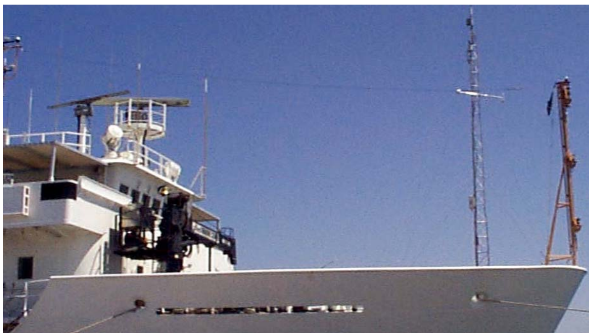
Figure S2. Guyed mast installed on foredeck for good exposure of meteorological instruments.
