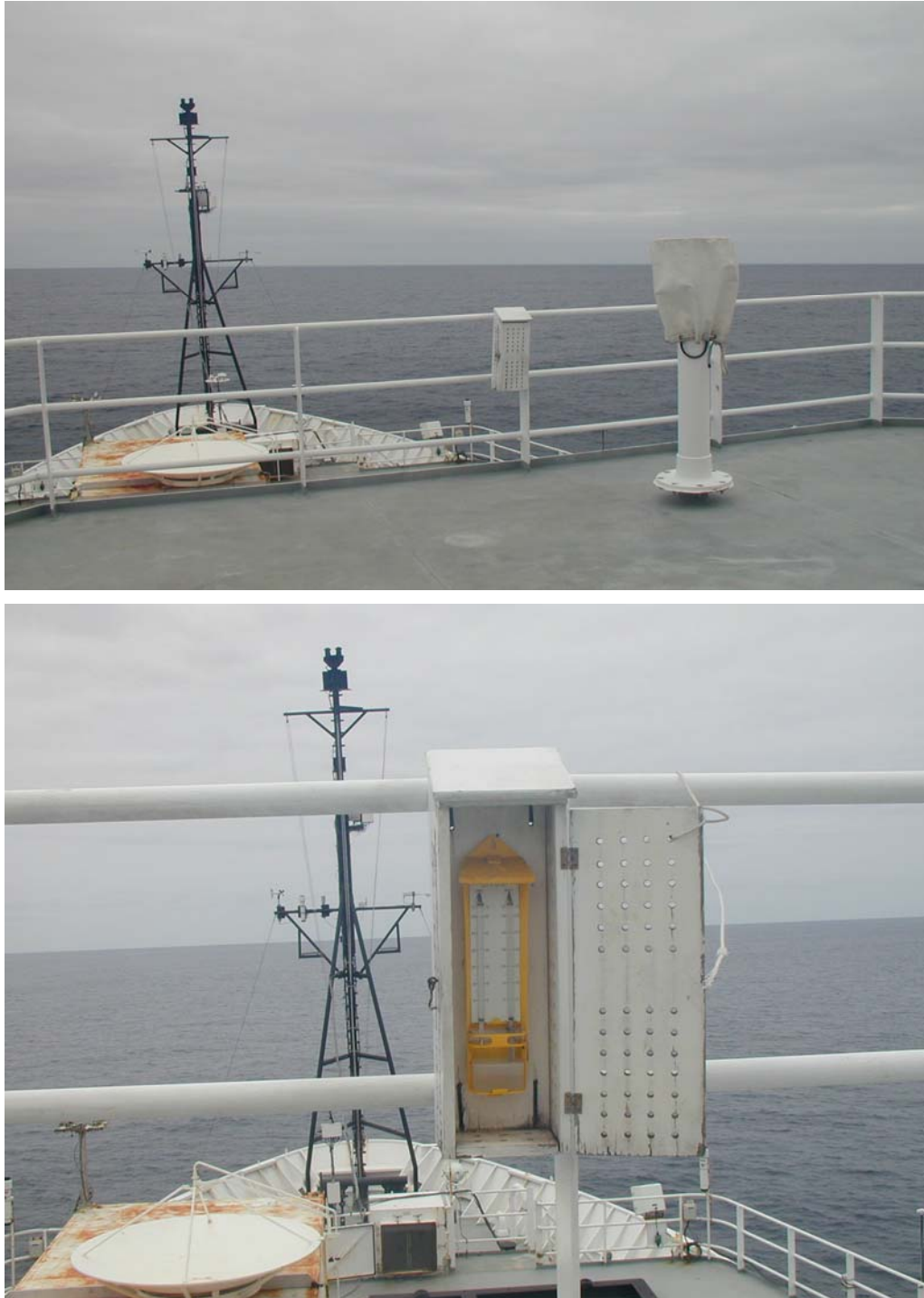
Figure 3.3. Example of the installation of wet and dry bulb thermometers used for the hourly weather observations transmitted to shore by ships participating in the Voluntary Observing Ships (VOS) program. This screen is in a well-exposed location, but the screen design is poor leading to inadequate ventilation of the wet and dry-bulb thermometers. In sunny conditions the temperature inside the box could be several degrees above ambient and the air-flow through the box is not sufficient for accurate measurement of the web-bulb depression. Observations from this unit during mostly overcast conditions are given in Figure 3.2.
