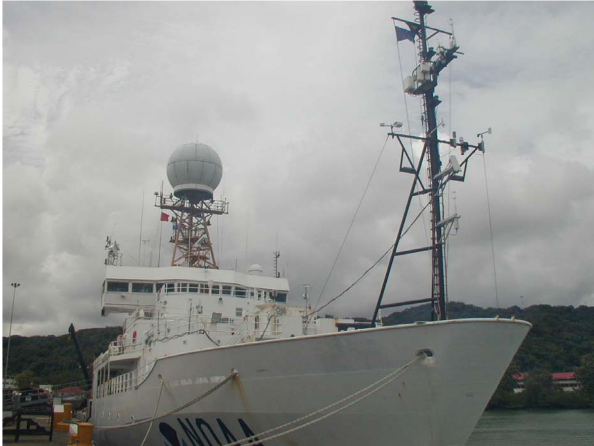
Figure 9.1 Meteorological instruments on the foremast of the NOAA ship Ronald H. Brown; a) below the upper crossarm is a covariance package. The sensor of the sonic anemometer is well exposed, although the instrument boxes below and behind it represent a greater obstacle to air flow than is desirable; b) closeup of the bulk flux instrument package. From left to right on crossarm: optical rain gauge; T/RH sensor with forced ventilation; second T/RH sensor in naturally ventilated screen; siphon rain gauge; propeller anemometer and wind vane unit. Below these instruments can be seen a laser wave-height sensor aimed forward of the bow and a second sonic anemometer.
