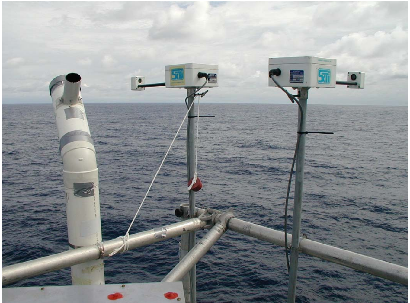
Figure 3.6 Example deployment of optical rain gauges. A pair of sensors is mounted with their axes oriented at 90^\circ to each other. This geometry helps with the wind correction procedure.
