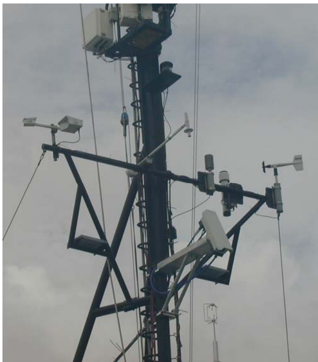
Figure 9.1 Meteorological instruments on the foremast of the NOAA ship Ronald H. Brown; a) below the upper crossarm is a covariance package. The sensor of the sonic anemometer is well exposed, although the instrument boxes below and behind it represent a greater obstacle to air flow than is desirable; b) closeup of the bulk flux instrument package. From left to right on crossarm: optical rain gauge; T/RH sensor with forced ventilation; second T/RH sensor in naturally ventilated screen; siphon rain gauge; propeller anemometer and wind vane unit. Below these instruments can be seen a laser wave-height sensor aimed forward of the bow and a second sonic anemometer.
