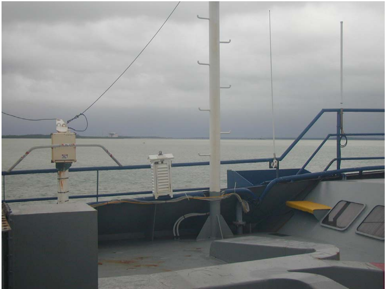
Figure 3.4. A more usual type of screen to house the wet and dry bulb thermometers read hourly by the bridge officers. It is also well-exposed, but all four sides are louvered to allow free air flow to the thermometers.
