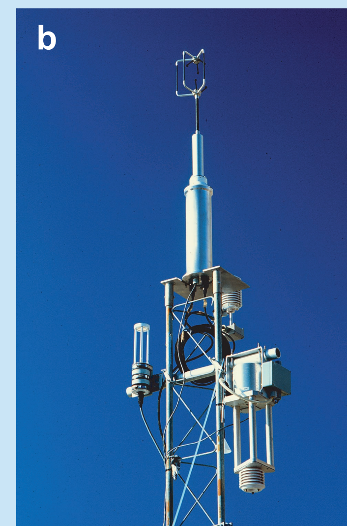
Figure 4: (a) R/V Roger Revelle and WHOI flux reference buoy. (b) PSD direct flux sensors. Photo credit: Chris Fairall.
