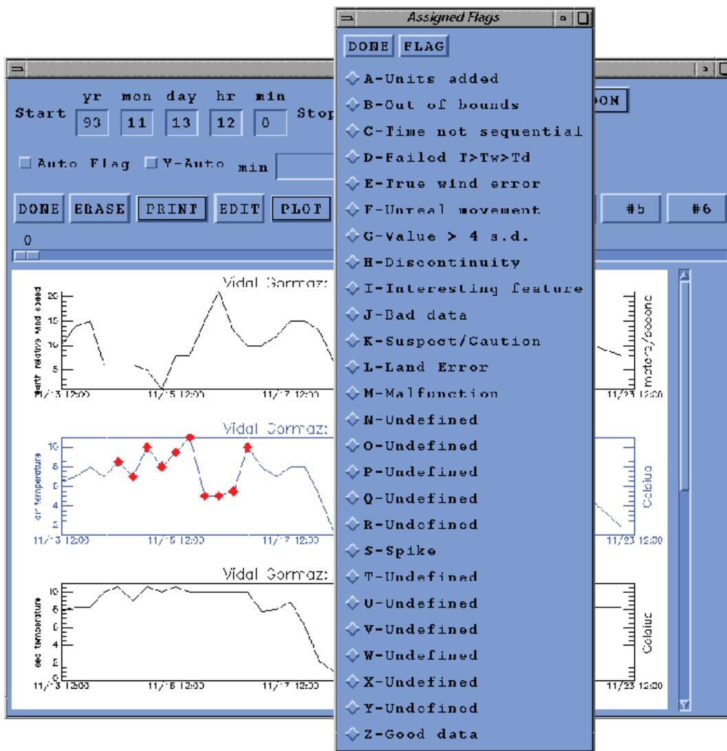
**Figure 12.** Screen shot of R/V *Vidal Gormaz* SR-01 data without flags displayed. The overlying window is a point and click flag selector used to flag the highlighted values.
