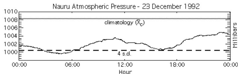
**Figure 2.** Atmospheric pressure data from the island of Nauru for December 1992 showing values that are greater than four standard deviations (dashed line) from the da Silva et al. (1994) mean (grey line).
