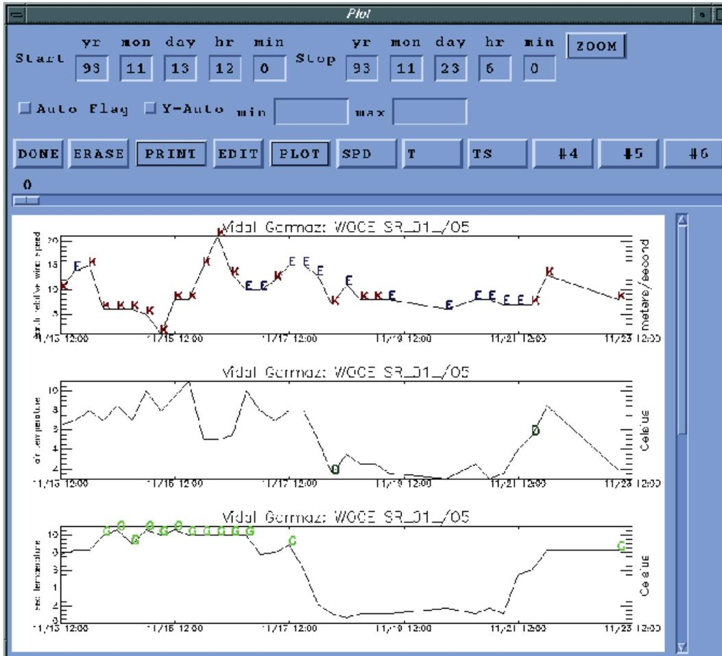
**Figure 11.** Screen shot of the VIDAT editor window with assigned QC flags displayed. Data for wind speed, air temperature, and sea temperature are shown for the 1993 SR-01 cruise of the R/V *Vidal Gormaz*
