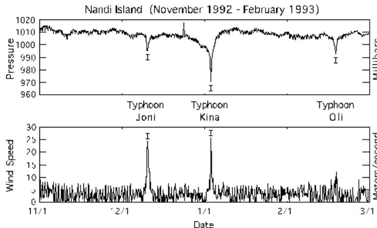
**Figure 14.** Typhoons Joni, Kina, and Oli passed the island of Nandi and were noted with the interesting feature flag *I*. Usually the *I* flag is applied to multiple variables, in this case atmospheric pressure and wind speed.
