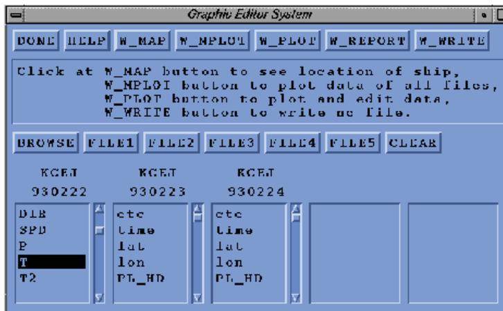
**Figure 8.** Screen shot of the file access window for the Visual Data Assessment Tool (VIDAT). The buttons across the top have drop down menu options. Three consecutive daily files from the R/V *Knorr* have been selected for review.
