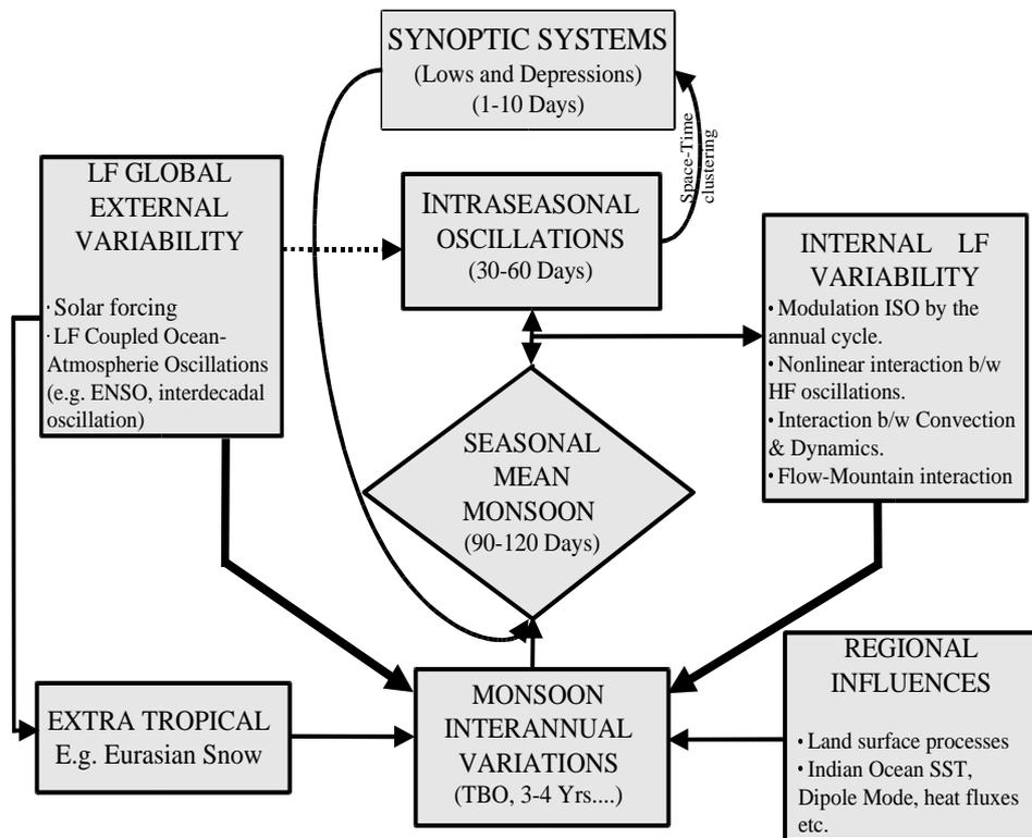
Figure 1.1. A schematic diagram indicating how monsoon ISO's influence the seasonal mean monsoon and its interannual variability by producing LF 'internal' variability through multi-scale interactions. Other 'external' forcing influencing the interannual variability of the monsoon are also indicated.
