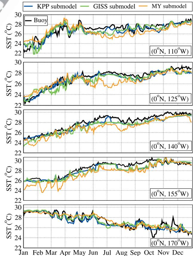
**Figure 5.** Daily SST time series from TAO buoys and those obtained from HYCOM simulations performed with three mixed layer submodels in 1997 when the El Niño started in April. HYCOM is forced using ECMWF wind and thermal forcing. No data, including SST, are assimilated by HYCOM for the simulations.
