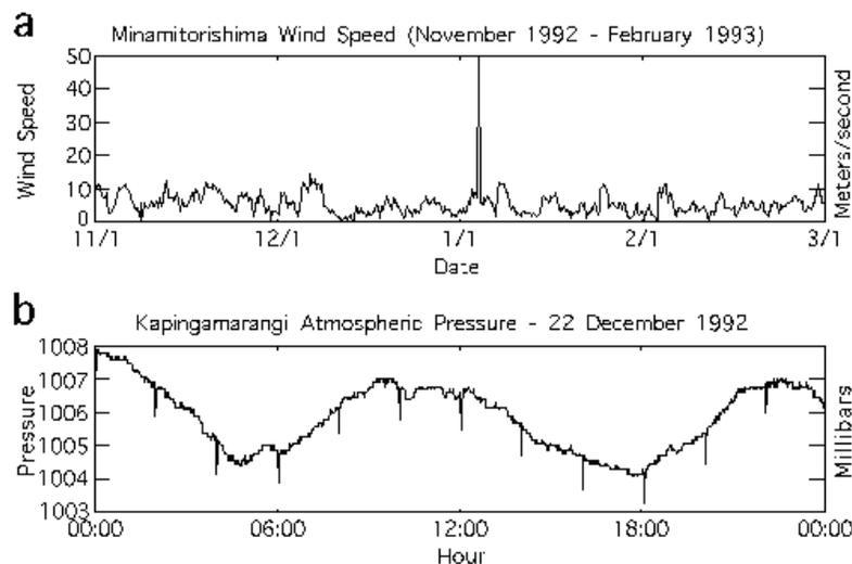
**Figure 17.** Examples of (a) a single large wind speed spike at Minamitorishima and (b) rhythmic one millibar atmospheric pressure spikes at Kapingamarangi. Both are flagged with an S.
