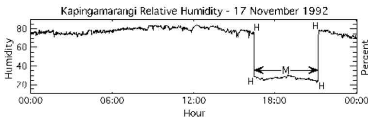
**Figure 13.** Discontinuity in the one-minute relative humidity data at the island of Kapingamarangi. The H flags are positioned at the starting and ending values of the discontinuity. In this case the discontinuity was caused by a sensor malfunction and all the values near 30% were flagged with an M.
