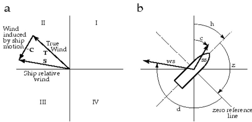
**Figure 6.** Schematic diagrams showing a) vector subtraction method of calculating the true wind and b) the six vectors and angles required to compute the true wind (T). In a) the roman numerals mark the quadrants in the cartesian coordinate system. (see text for more details)
