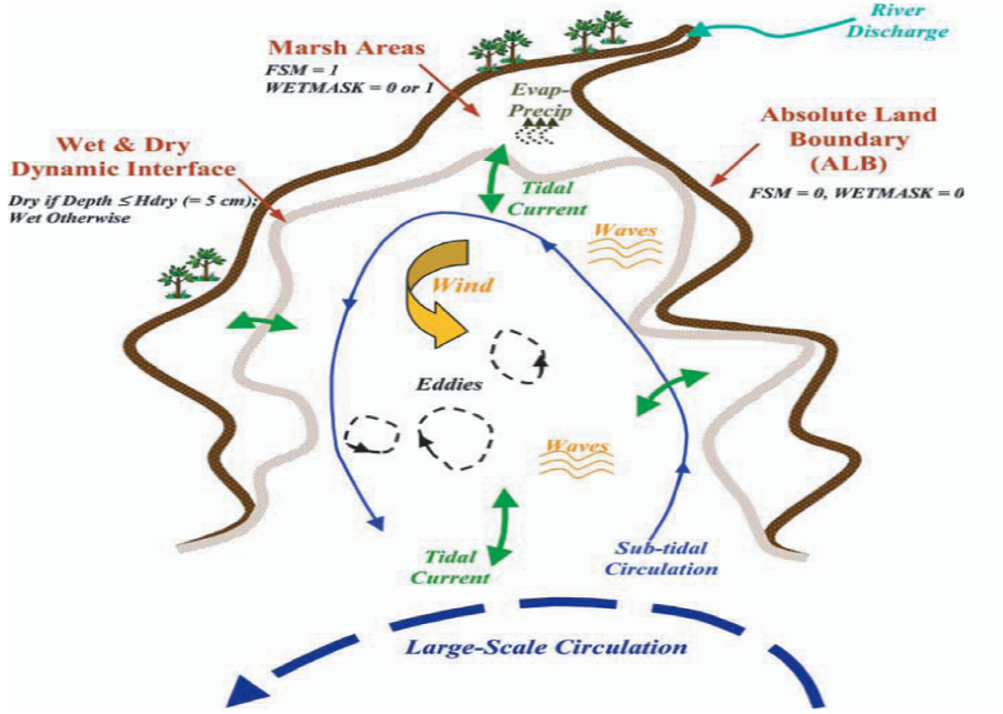
Figure 5: Schematic of a coastal ocean region that can be flooded and drained (dried) by water-level variations from the open ocean (from Oey , 2004).
